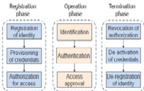
Fig.1 Phases of IDM and access control
