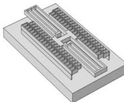
Fig.2. Electrostatically driven comb actuator
