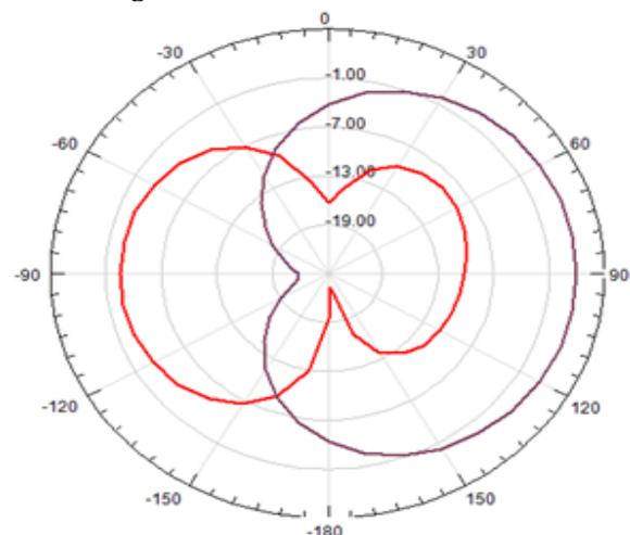
Figure 5. Radiation Pattern of proposed antenna at Phi=0 and 90 degree
