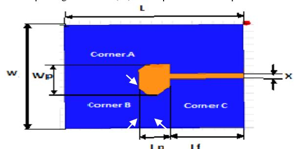
Figure 1. Geometry of proposed antenna showing patch and substrate
