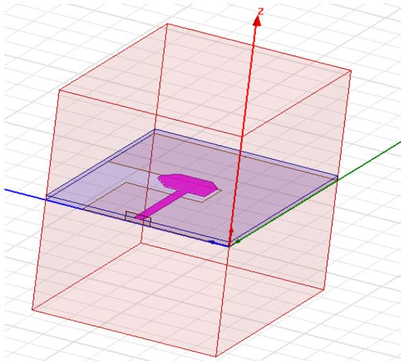
Figure 2. 3D Ansoft HFSS generated model of proposed antenna
