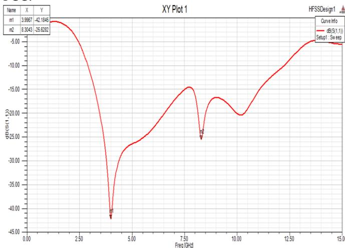
Figure 3. Return Loss of the Proposed Antenna
