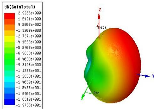
Figure 6. 3-D Polar Plot Showing Total Gain (in dB)
