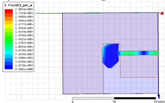
Figure 9. E- Field Distribution of proposed antenna
