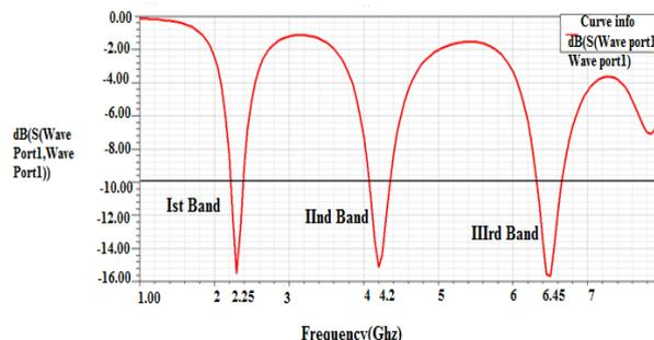
Figure 3.3 S11 Parameter of Sierpinski Prefractal antenna
