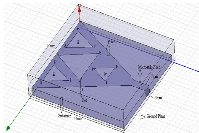
Figure 3.2 Isometric view of Prefractal Sierpinski antenna
