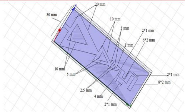
Figure 2 Top view of antenna
