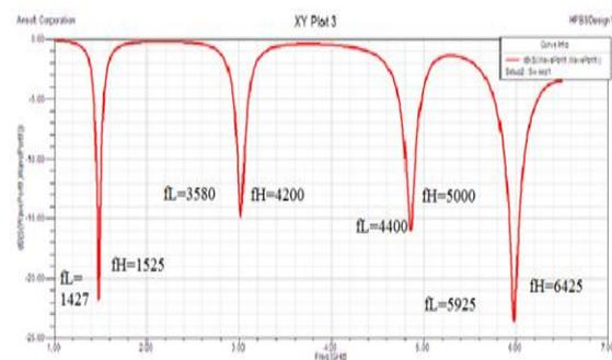
Figure 3 Return loss of antenna
