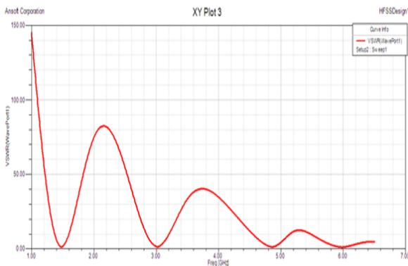
**Figure 4 VAWR of antenna**
