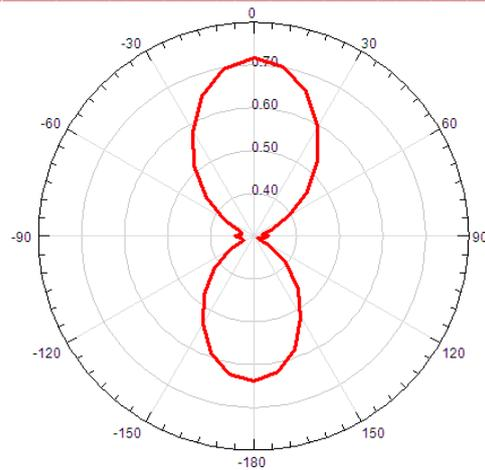
**Figure 6 Radiation pattern of antenna**
