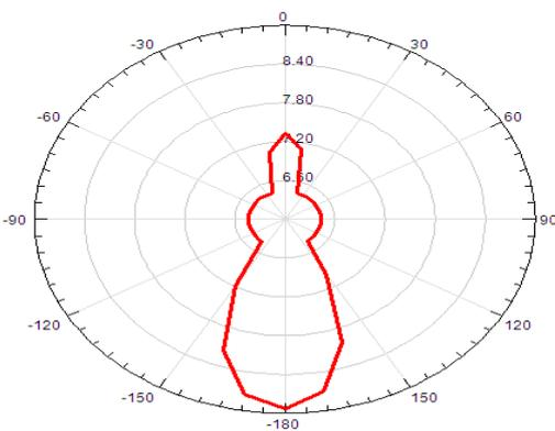
**Figure 5 Radiation pattern of antenna**
