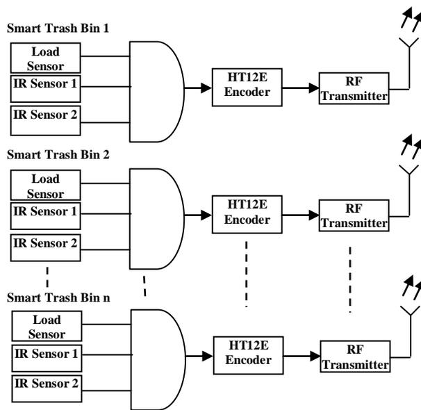
Fig 2: Smart Trash System
