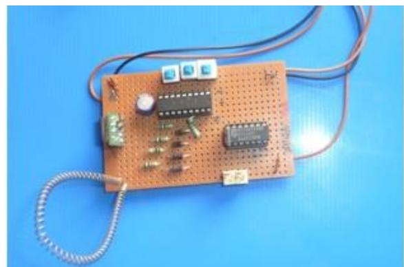
Layout of RF Transmitter Module
