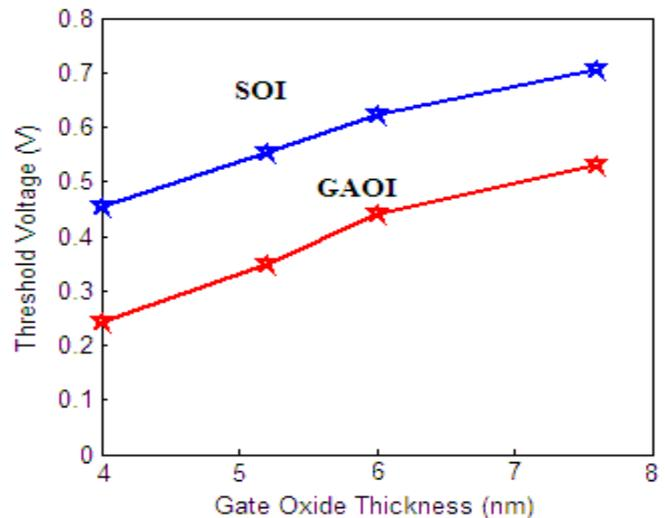
Figure 2 Threshold voltage with gate oxide thickness for a channel length 90nm
