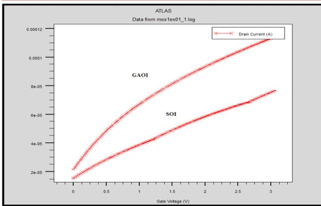
Figure. 4 Drain current with gate voltage for gate oxide Thickness 5nm and channel length 90nm
