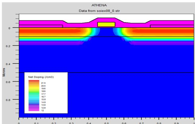
Figure 1 ATHENA simulated SOI structure and for GAOI the channel Silicon material has been replaced with GaAs
