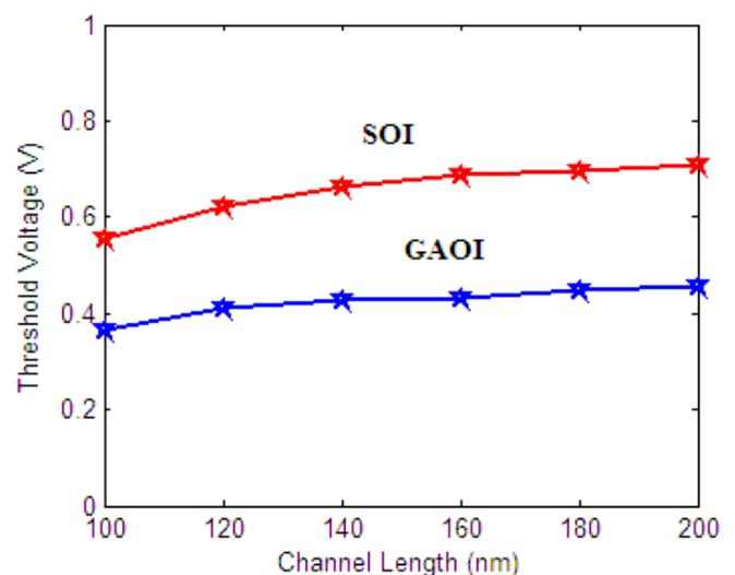
Figure. 3 Threshold voltage variation with channel length for gate oxide thickness 5nm
