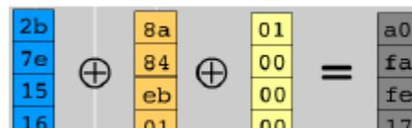
The second column is generated by XOR-ing the 1<sup>st</sup> column of the i<sup>th</sup> key with the second column of the i-1<sup>th</sup> key.
