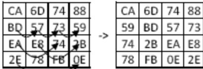
d) Inverse Sub Bytes – This step replaces each entry in the matrix from the corresponding entry in the inverse S-Box[2] as shown in figure.
