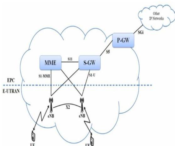
Figure 1.1: LTE- Advanced Network Architecture
