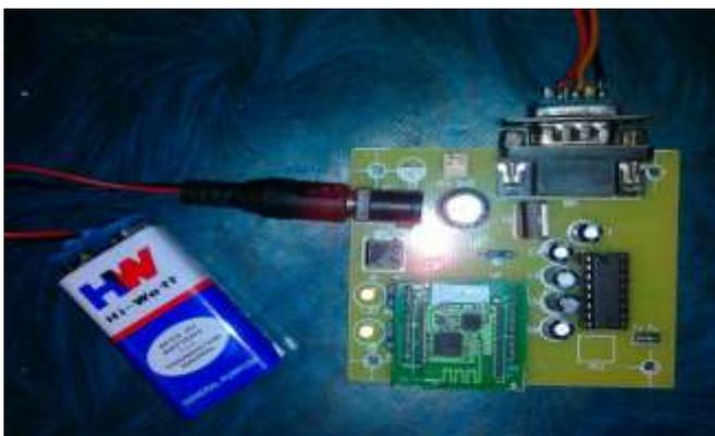
Fig 6: photo of zigbee module
