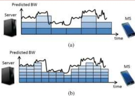
Fig.2. svc Layer System (a) Traditional video streaming (b) Svc layers, scalable and adaptive streaming Concern the mobile user side or the link quality. If some packets are lost, then also mobile user can decode the video. Hence SVC-based video streaming at the server side needs to be controlled with the rate adaptation method for efficiently utilizing the bandwidth. The SVC video streaming have flexible scalability, and high quality coding efficiency.
