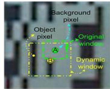
Fig. 8 Dynamic-sized Window centering the nearest Edge pixel[1]
