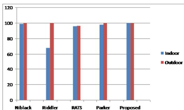
Fig. 16. Graph Recognition rates for the barcode images binarized using DWE strategy evaluated using by choosing different window sizes and evaluated using (zxing decoder)
