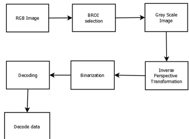
Fig. 9 Data flow Architecture
