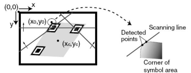
Fig. 6 Three scanning lines are used for the corners detection. [2]
