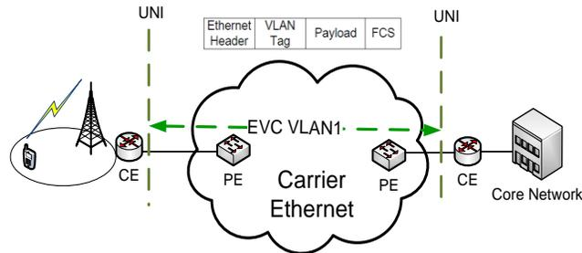
Figure 2. Generic Carrier Backhaul Architecture
