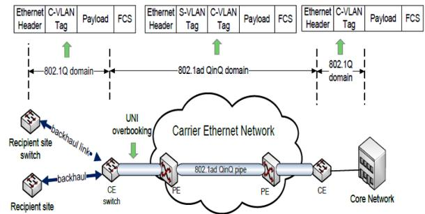
Figure 4. Q-in-Q Tunneling Carrier Backhaul Architecture
