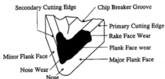
Fig.1. Wear zones on the cutting tool caused by chip formation [3]
