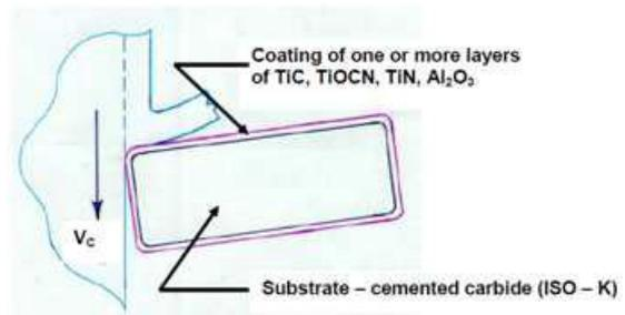
Fig. 2 Machining by Coated Carbide Insert
