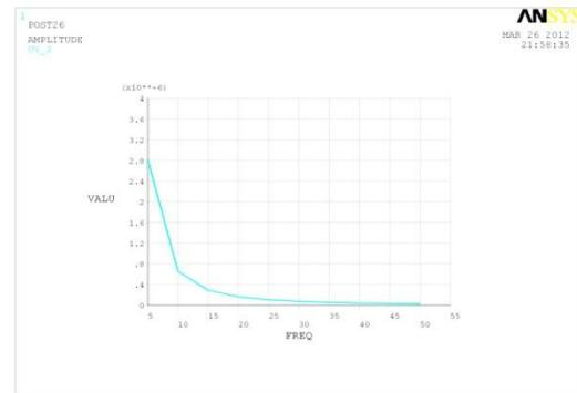
**Fig 21: Figure showing the reduction of vibration for FG 400 material for 3D**
