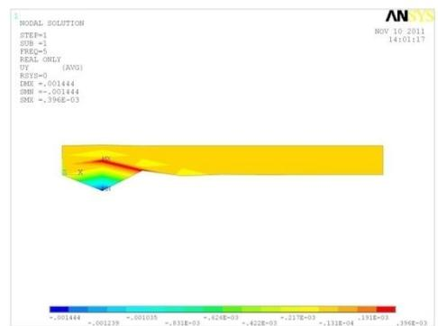
Fig13: Nodal solution for 70 bar compression pressure (FG 260)
