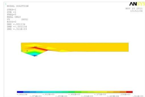
Fig7: Nodal solution for 55 bar compression pressure (FG 260)
