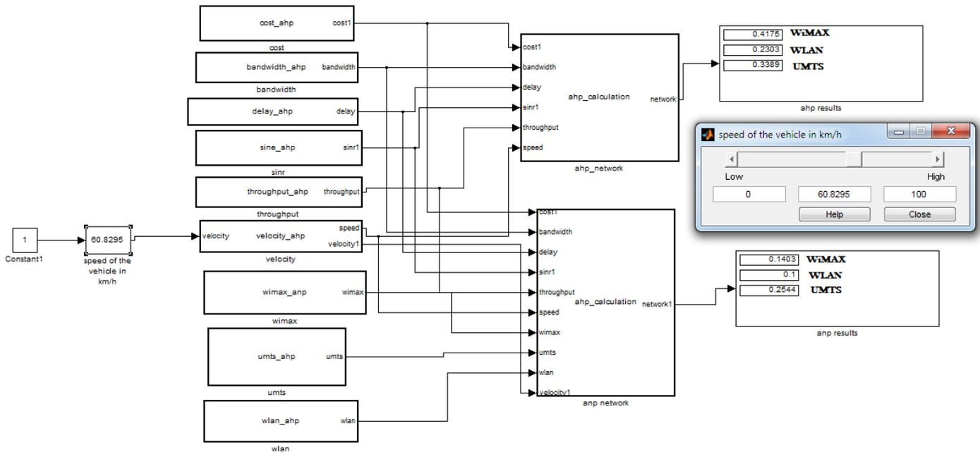
Figure 4. SIMULINK model for ANP and AHP based Vertical Handover.
