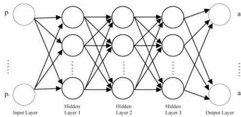
Figure 3. Feed Forward Backpropagation Neural Network with 5 layers
