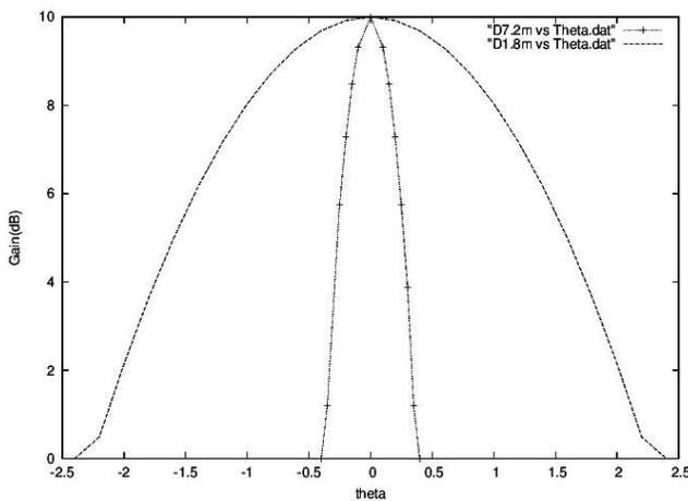
Figure-7 Gain (dB) for 7. 2m diameter antenna and 1. 8 diameterantenna verses  $\theta$
