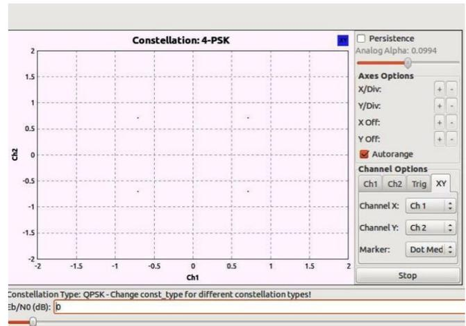
Figure-3 Scatter diagram plot of QPSK transmitter
