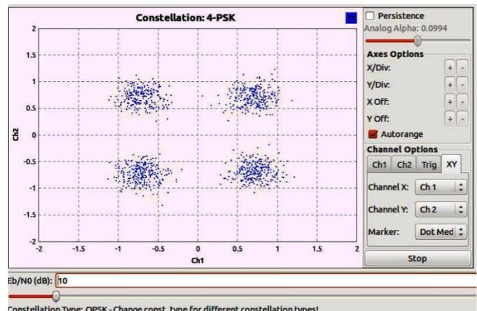
Figure-4 Scatter diagram plot of QPSK receiver
