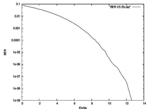
Figure-5 Bit Error Rate(BER) of simulated model
