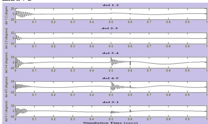
**Fig.2 Plot of Relative Rotor Angle with Time of MM System with SVC**
