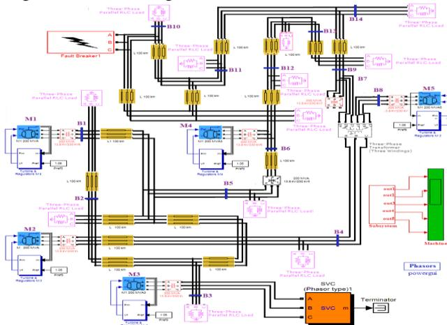
**Fig1 SIMULINK Model of Multi-Machine System with Fault and SVC**
