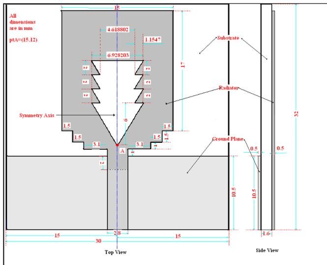
Figure 1: Geometry of proposed Microstrip antenna.
