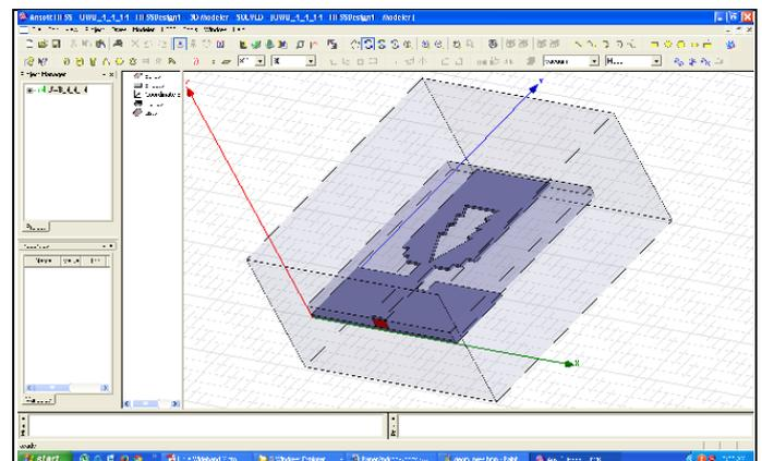
Figure 4: Prototype of proposed antenna designed in HFSS v11.0
