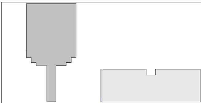
Figure 2: Separate view of radiator (left) and ground plane (right).
