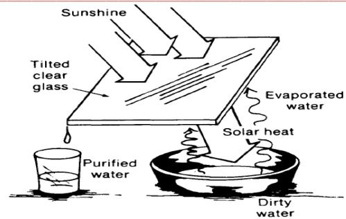
Figure 2: Basis concept of solar distillation [3]
