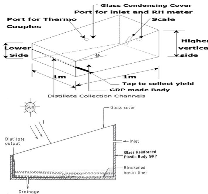
Figure 5: Conventional type solar still with GRP body [14]
