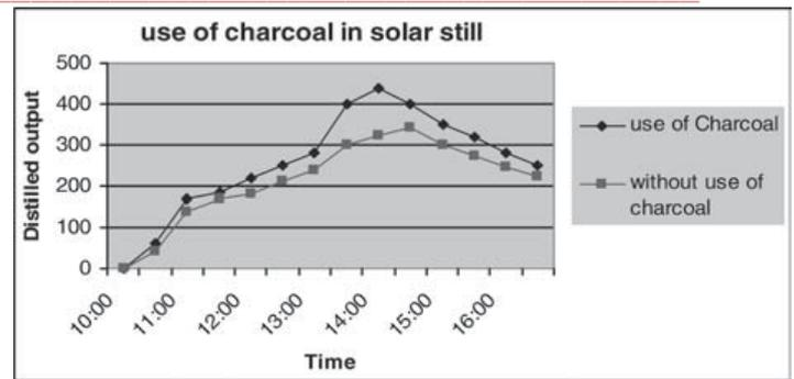
Figure 4: Use of Charcoal as Energy Absorbing Material
