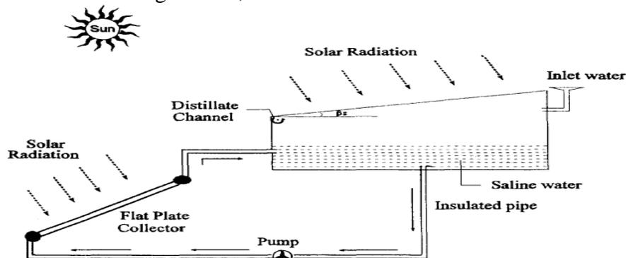
Figure 3. Schematic view of an active solar still coupled with a flat plate [8]
