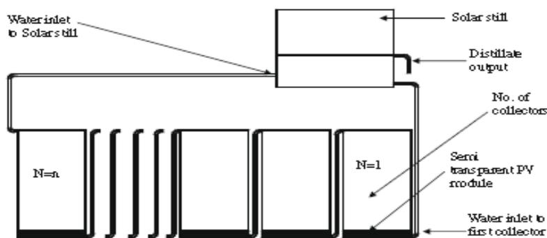
Figure 2. Schematic diagram of PV/T collectors connected in series [7]
