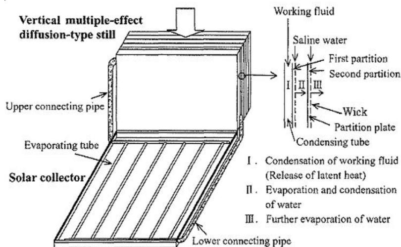
Figure 5. Schematic diagram of vertical multiple-effect diffusion-type still coupled with a heat- pipe solar Collector [10]
