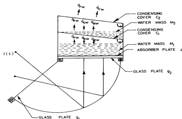
Figure 3. Schematic view of an inverted absorber double basin solar still [11]
