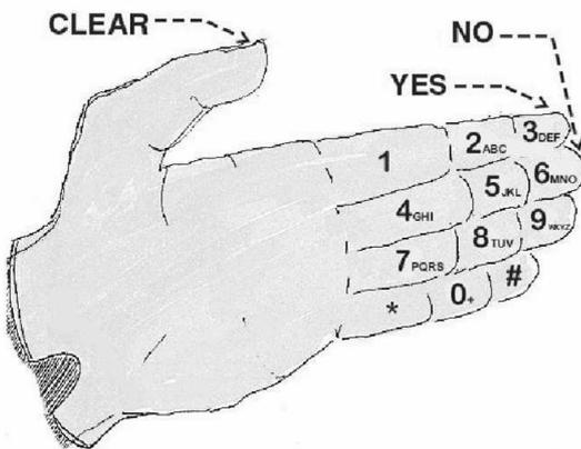
Figure 2. Finger-joint Gesture Wearable Keypad[18]
