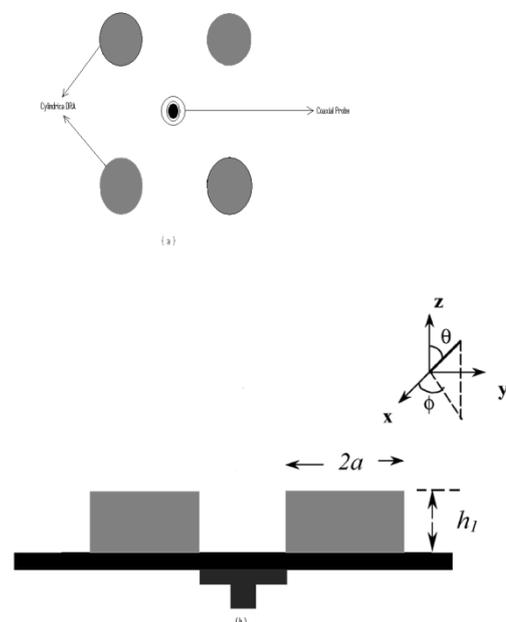
Fig.1 Four-element Cylindrical DRA fed by a coaxial probe.
