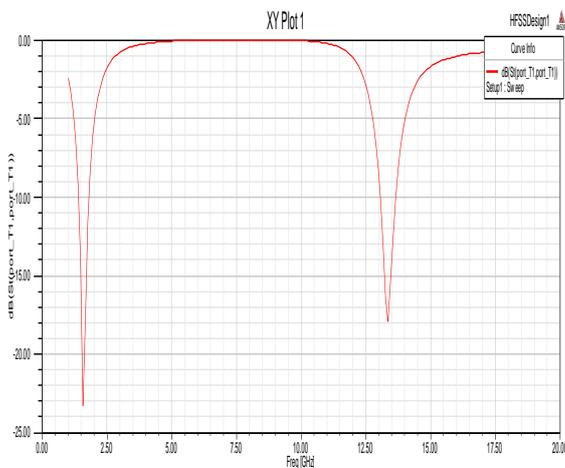
Fig.2 Return Loss for the four element cylindrical shaped dielectric resonator antenna
