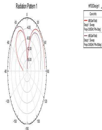
Fig.6 Radiation Pattern for a four element cylindrical dielectric resonator antenna by top loading with a thin circular disc of radius 7 mm and height 1.65 mm.
