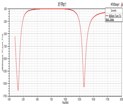
Fig.9 Return Loss for a four element cylindrical dielectric resonator antenna by top loading with a thin circular disc of radius 7 mm and height 1.00 mm
