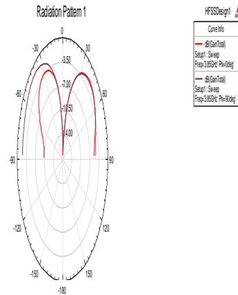
Fig.10 Radiation Pattern for a four element cylindrical dielectric resonator antenna by top loading with a thin circular disc of radius 7 mm and height 1.00 mm
