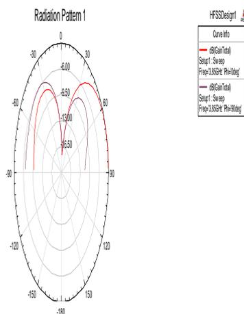
Fig.3 Radiation Pattern for the four element cylindrical shaped dielectric resonator antenna
