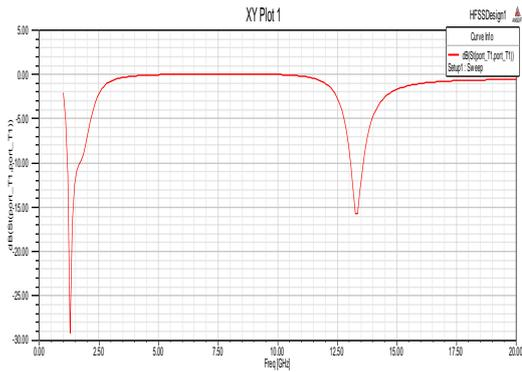
Fig.7 Return Loss for a four element cylindrical dielectric resonator antenna by top loading with a thin circular disc of radius 7 mm and height 1.05 mm.
