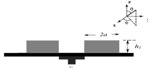
Fig.4 Cross-Sectional view of Four-element Cylindrical DRA by top loading a thin circular disc
