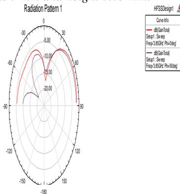
Fig.8 Radiation Pattern for a four element cylindrical dielectric resonator antenna by top loading with a thin circular disc of radius 7 mm and height 1.05 mm
