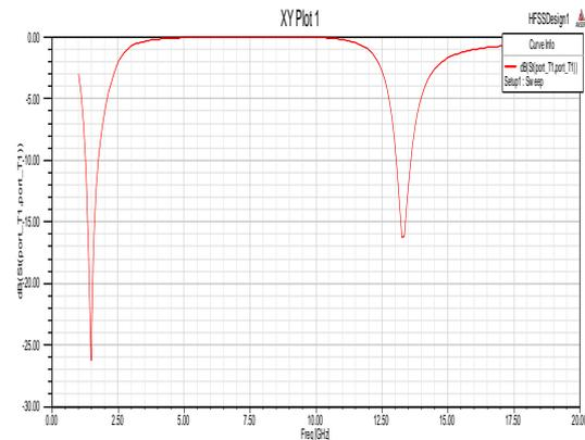
Fig.5 Return Loss for a four element cylindrical dielectric resonator antenna by top loading with a thin circular disc of radius 7 mm and height 1.65 mm.
