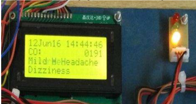
Fig.3:Real time alerts on LCD
