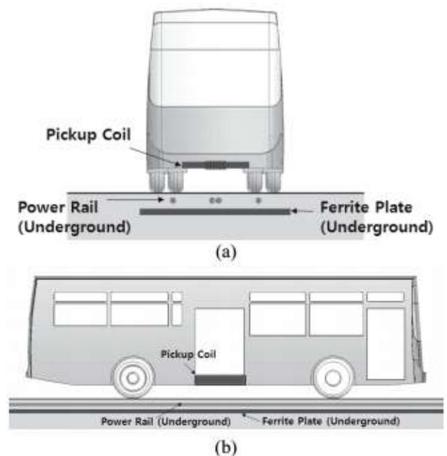
**Fig. 1** OLVE and its power transfer system: (a) side view and (b) front view
