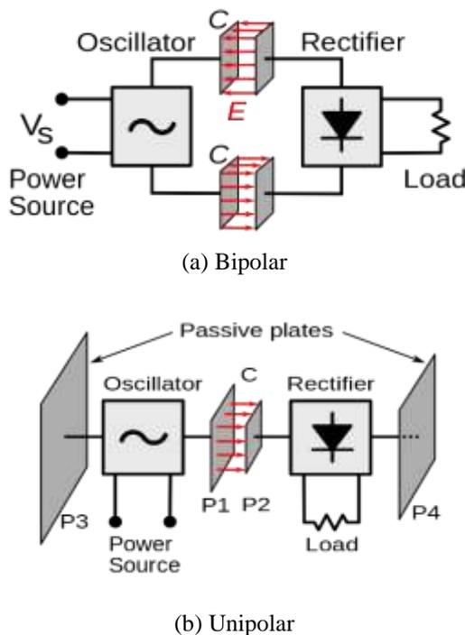
Fig. 2 Capacitive wireless power system
