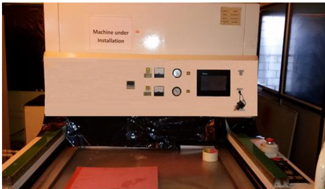
Figure 2 PLC based Exposure Machine for PCB fabrication
