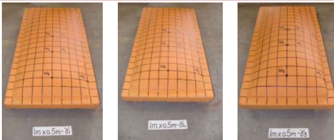
Fig.2.4 Shell specimens with various rises
