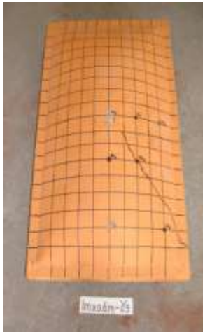
Fig. 3.3 Crack patterns of shell specimens
