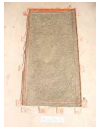
Fig.2.3 Casting of shell specimen
