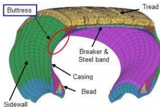
**Figure 4. 3D Finite Element Model**
