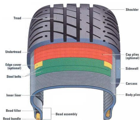
Figure 2. Constructional features of tire
