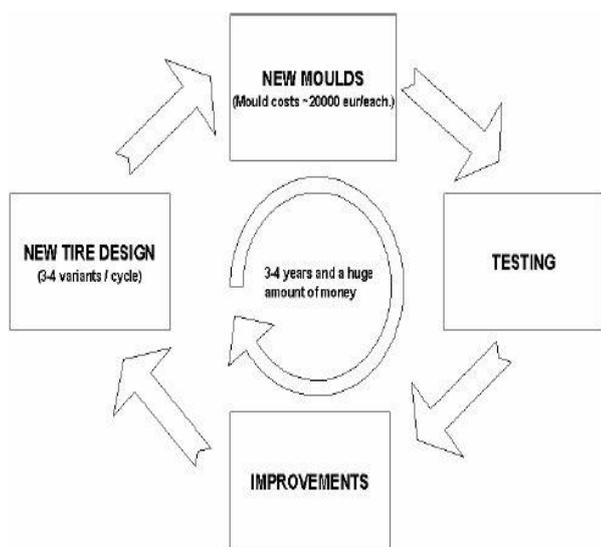
Figure 1. Traditional tire R&D process
