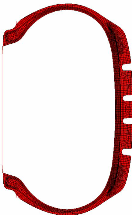
**Figure 3. Axisymmetric FE-model after inflation**
