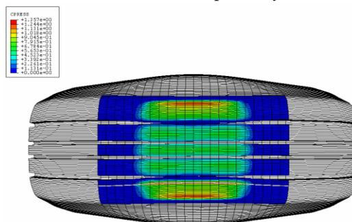
**Figure 5. 3D Footprint result of Tire**
