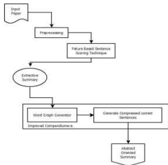
Figuter.1: System Architecture
