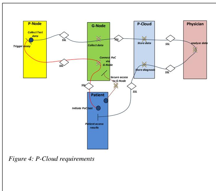
Figure 5 shows the UCM representation of the PoC system indicating all the P-Cloud requirements stated. A similar approach is shown in reference [13]. The responsibilities (or the functionalities) required within each domain are displayed as 'X'. The diamond indicates the SSL connectivity between all the players in the data collection to data storage.
