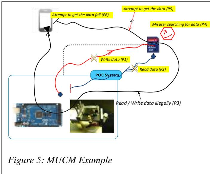
Figure 6 shows the UCM and the MUCM paths for accessing data from and to the SD card. Since the initial data storage is the SD card, the data on the SD card must be protected. The path P1 in the figure is a normal operation for writing data to the SD card during the test. Path P2 shows, reading data from the SD card. These are the UCM representation for R/W data from/to with respect to the SD card.
