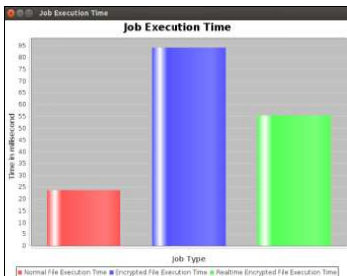
Figure 7: Shows graph of comparison of job execution time of original file and files after encryption using AES and Real Time encryption algorithm
