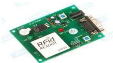
Figure 4. 125KHz RFID Reader Module
