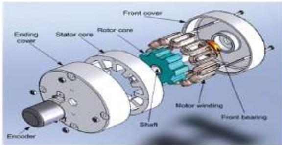
Fig.3. Construction diagram of SRM
