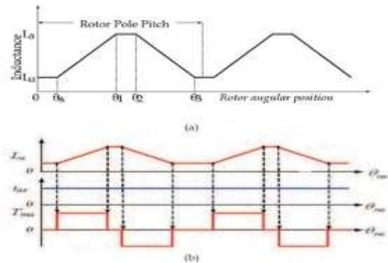
Fig. 2 (a) Inductance and (b) torque in SRM
