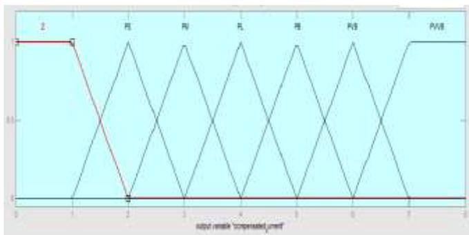
Fig. 12 Membership functions of Compensated Current
