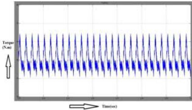
Fig. 22 Toque waveform with PI controller
