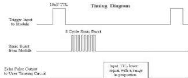
Fig 4 Timing diagram of ultrasonic sensor.
