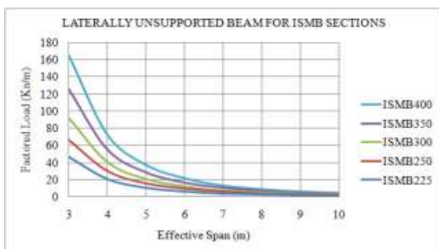
Fig.13 Factored load vs. effective span for laterally unsupported ISMB beams
