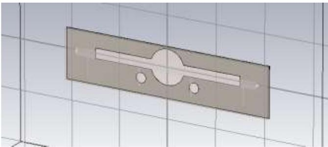
Figure 4: Back View of Proposed 4<sup>th</sup> order HPF using DGS.
