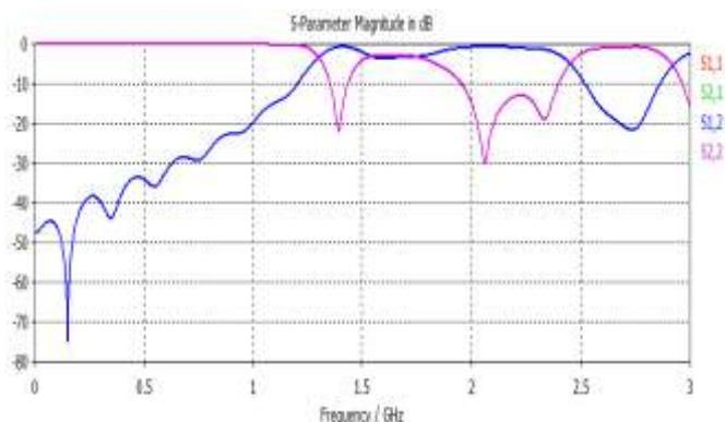
Figure 5: Simulated results of proposed HPF using DGS
