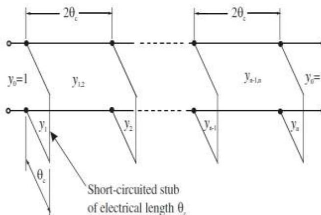
Figure 1: Optimum distributed high pass filter
