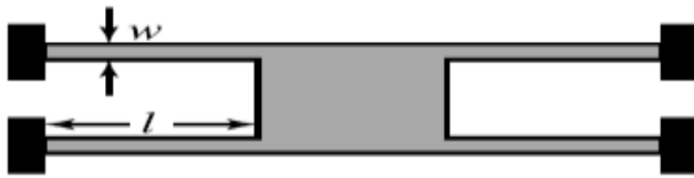
Fig.2 Fixed-fixed flexure beam
