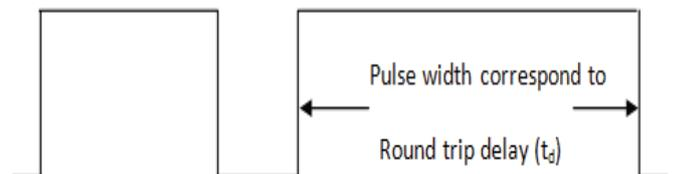
Fig. 5.1 Ultrasonic sensor output wave
