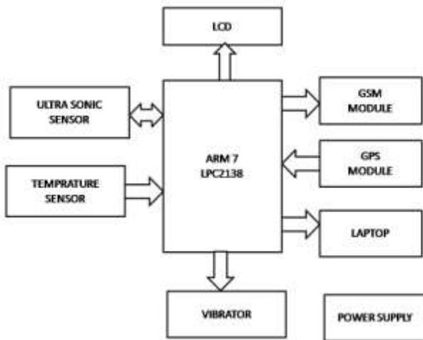
Fig. 5.2 Hardware Block Diagram
