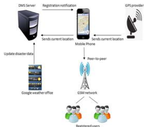
Figure:1 Proposed location based early disaster warning and evacuation system
