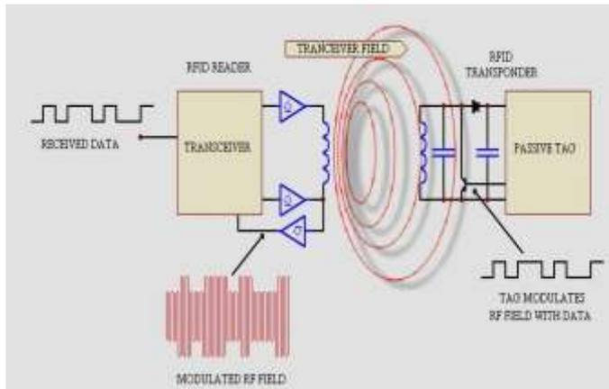
Figure. 1. Example of RFID System [8]
