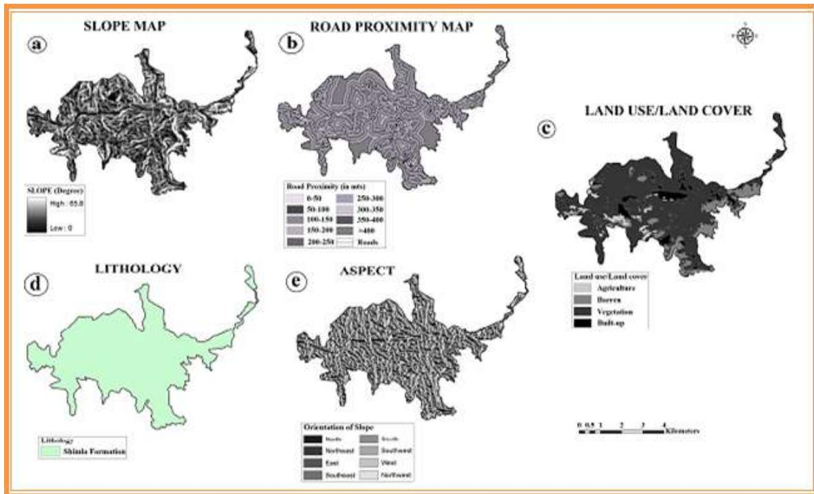
**Fig.3. (a) slope (b) road proximity(c) land use (d) lithology (e) aspect [1]**
