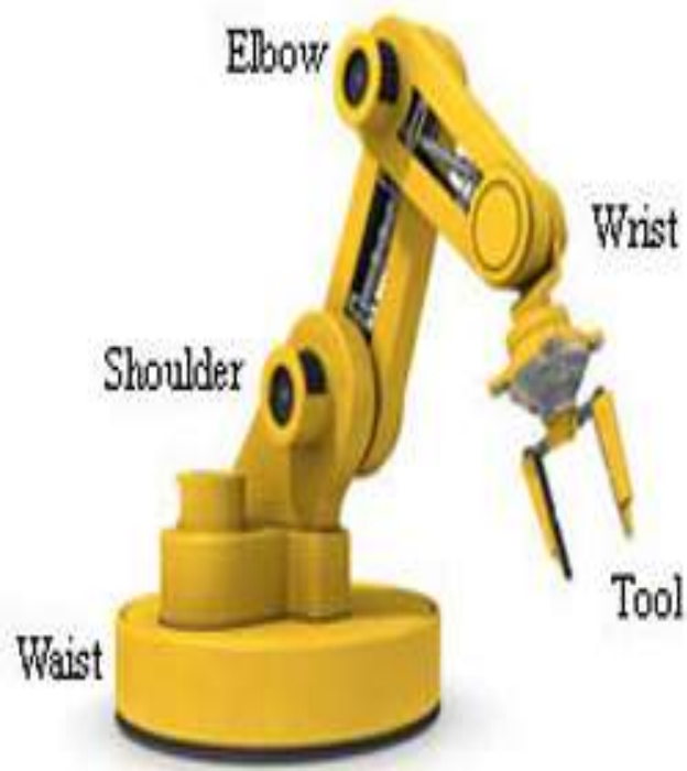
Figure 8: Mechanical movement of robotic arm
