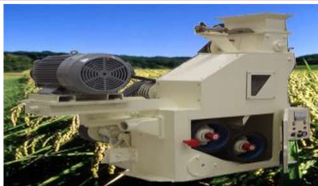
Figure 8.Modern automated rice husking machine.
