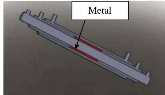
Fig 2 Sectional view indicating Location of metal foam
