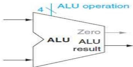
Figure 6 : Arithmetic Logic Unit
