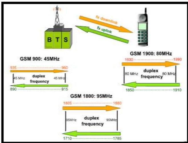
Fig.1. GSM FDD structure
