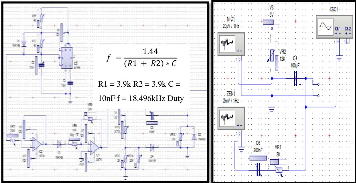
Fig. 4(a). Intermediate frequency circuit
