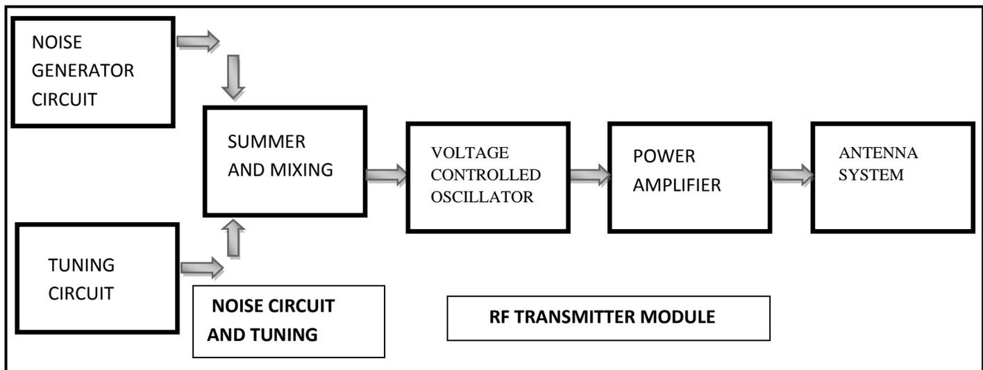
Fig. 3. Block diagram of Mobile phone jammer
