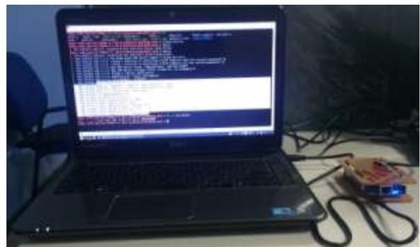
Figure 3. BeagleBone Connected to Linux PC
