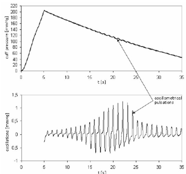
Figure 2: Conventional oscillometric graph for pressure and oscillation signal
