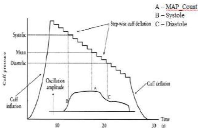
Figure 5 : Oscillometric curve
