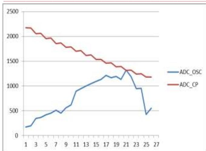
Figure 6 : ADC value of osc and cuff pressure plotted
