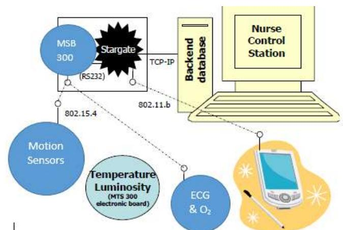
Fig 5: Monitoring system at Nurse Control station.
